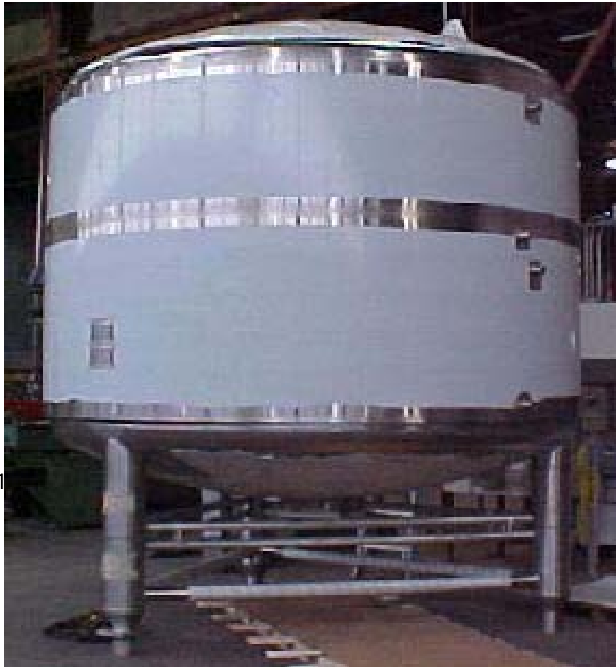
Vertical Vessel - Jacketed
